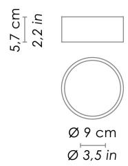
A collection of wall and ceiling lamps with a matt white or black painted die-cast aluminium fixture, a white polycarbonate diffuser and a LED light source.
